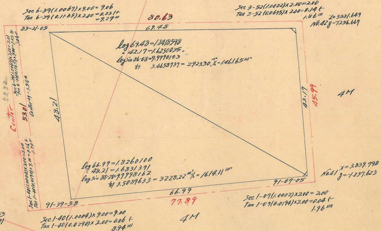
合計面積 =  $1.4616511 \text{ m}^2 + 1.61411 \text{ m}^2 = 3075.76 \text{ m}^2$  ( $\times 0.3025 = 930.41 \text{ m}^2$ ) =  $930.38 \text{ m}^2$
