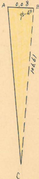
$\Delta ABC \text{ 面積} = \frac{1}{2} \times 0.08 \times 106.61 \times \sin 95-43 = 4.243 \text{ m}^2$
