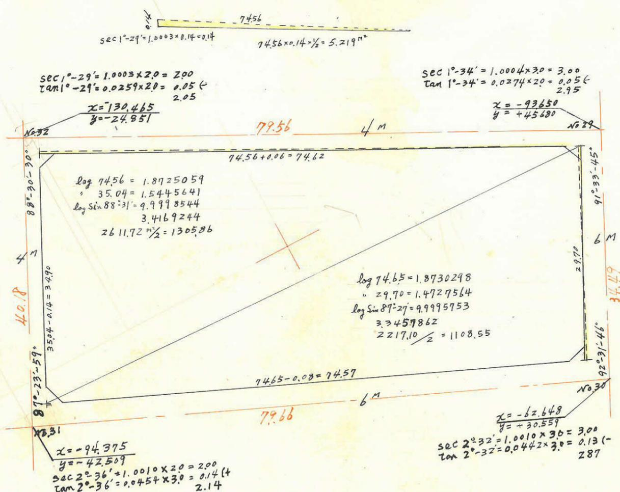
$$\begin{aligned} \log 74.56 &= 1.8725059 \\ 35.04 &= 1.5445641 \\ \log \sin 88^\circ-31' &= 9.9998544 \\ 3.4169244 \\ 2611.72 \text{ m}^2 &= 1305.86 \end{aligned}$$
