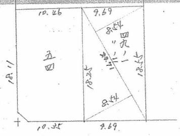
$$\left. \begin{array}{l} 49の1 \\ 49の2 \end{array} \right\} \frac{1}{2} 20.71 \times (8.54 + 8.54) = 176.8634 \text{ ㎡}$$
